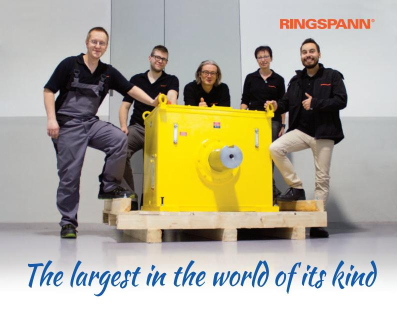
A few days ago, RINGSPANN completed the world's largest housing freewheel in technological history for an Asian client. It is the latest member of the FH series and is used in the energy recovery system of a petrochemical plant. As a wear-free overrunning clutch it generates a maximum nominal torque of 81,850 Nm at 1,400 rpm. With this innovative new development, RINGSPANN is entering completely new dimensions in freewheel technology and is once again setting international standards.
