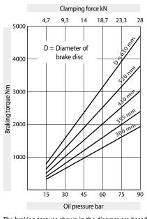
The braking torques shown in the diagram are based on a theoretical friction coefficient of 0,3.
